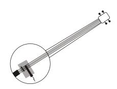
**Banjo:** Depending on the type of instrument and the style of play, the C-ducer can either be mounted with the adhesive foam pad stuck to the rim and just the tape portion attached to the skin. When percussive effects are used (ie tapping the skin) the position of the *tape* will alter the level of the effect.
